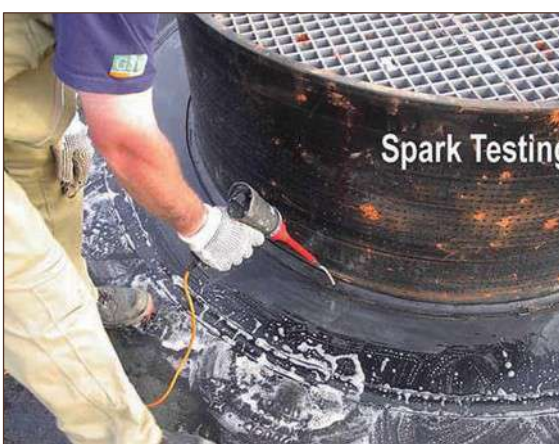
Figure A4.45 Spark testing (courtesy GSE Environmental)
