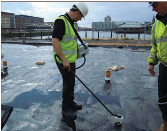
Figure A4.41 Small sand bags are marking holes made in the gas membrane used to check whether injected CO 2 has worked its way beneath whole area (courtesy Landline Ltd)
